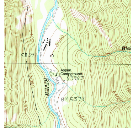
Figure 12.3: A topographical map displays elevation by drawing contour lines, along with the elevation is constant. Sample taken from the public domain USGS Digital Raster Graphics, http://topmaps.usgs.gov/drg/ .
